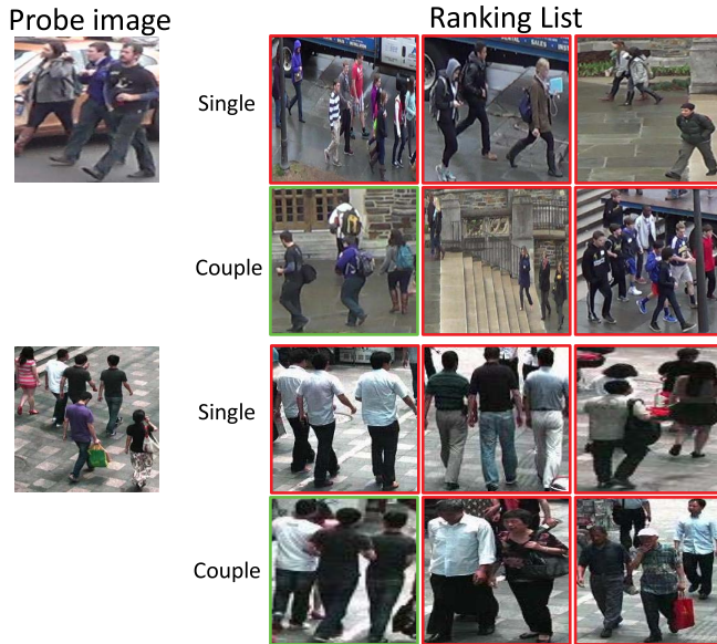
Fig. 7. Two visual examples showing the effectiveness of couple representations. These two examples are selected from the results of DukeMTMC Group and Road Group , respectively. The first column shows the probe image. The following columns show the top three matches. The samples highlighted by red bounding boxes indicate the negative results, while those highlighted by green bounding boxes indicate the positive results. ‘Single’ and ‘Couple’ represent that the results are obtained respectively by the single or couple representation learning. These two examples show that, in some cases that the single representations lose their effectiveness, the couple representations take their responsibility and offer better predictions.
