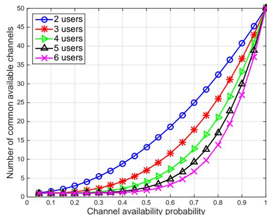
Fig. 2: The expected number of common available channels as a function of the channel availability probability and the number of users.
