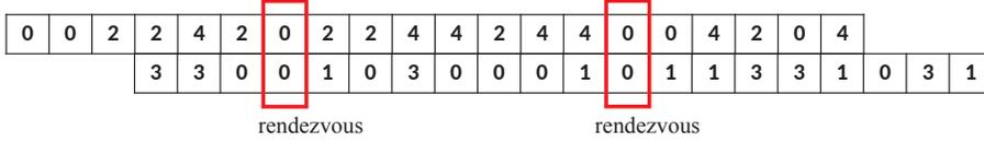
Fig. 1: An illustrating example for the two-prime modular clock algorithm with two users (the top sequence for user 1 and the bottom sequence for user 2).
